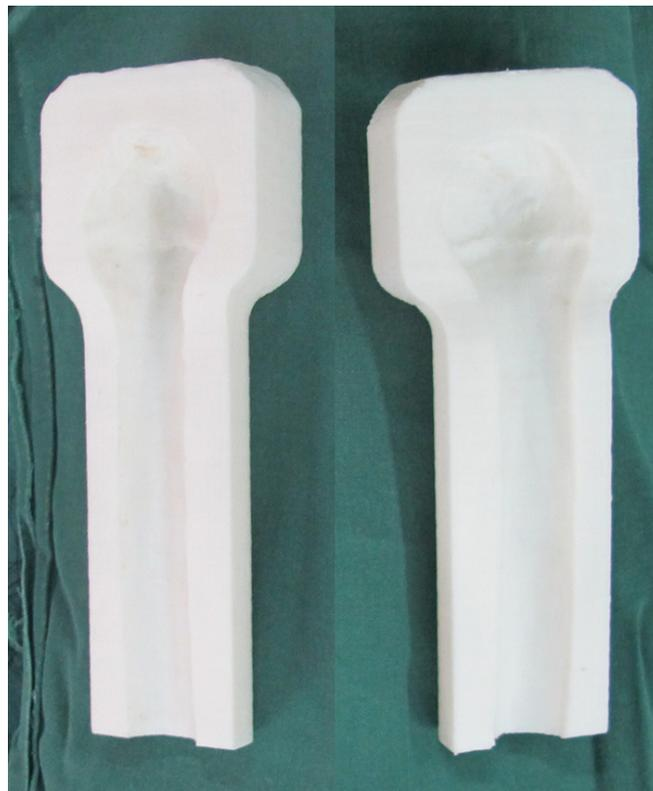
Fig 2 A photograph shows 3D-printed moulds, which were designed as two pieces in order to extrusion and separation the bone cement spacer easily when solid.
